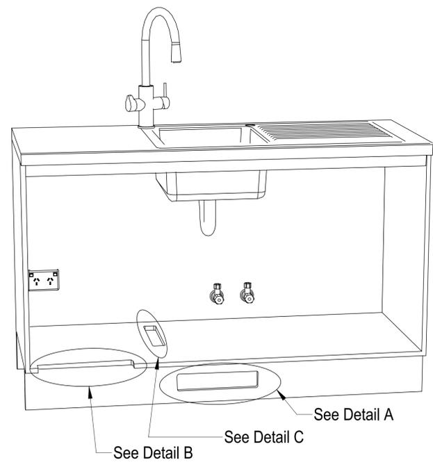
Position the Tap such that it dispenses into the sink bowl with ample clearance for a cup or a tea pot
