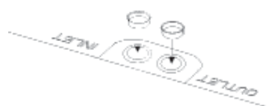
Figure 7 Close up view of the chiller water connections.
